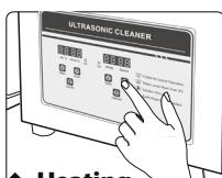
To start the device, you need to set the ultrasonic working time. Press the "Time+" button once to increase the working time by 1 minute and "Time-" to decrease the time by 1 minute. After setting the desired time, use the on/off button - the washer will start working and stop working after the set time.
