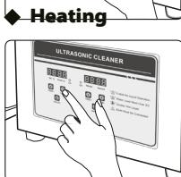
To activate the heating function, set the desired temperature. Press the "Temp+" button once to increase the temperature by 1st C and "Temp-" to decrease the desired temperature by 1 st C. After setting the desired temperature, use the on/off button. The heater will start operating and turn off when the desired temperature is reached
