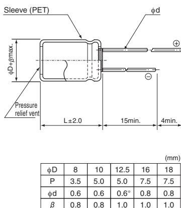
※ In case L &gt; 25 for the φ12.5 dia. unit, lead dia. φ d = 0.8mm.
