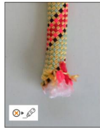
• Damaged rope end
