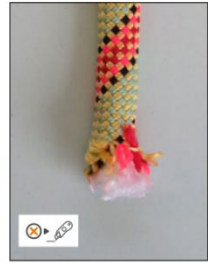
• Damaged rope end
