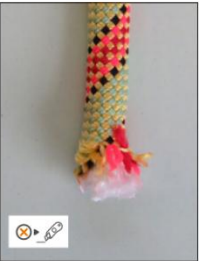
• Damaged rope end
