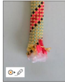
• Damaged rope end
