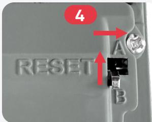
Move the RESET switch up and right from position „B“ back to position „A“.
