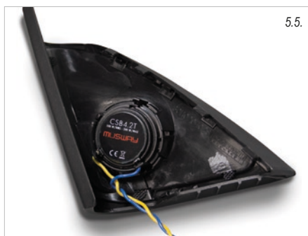
Plug the Musway tweeter into the mirror triangle
