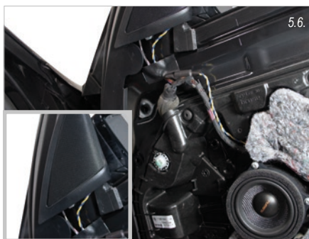
Attach the triangle to the door and connect the tweeter cable (See page 3 or Figure 5.3.)
