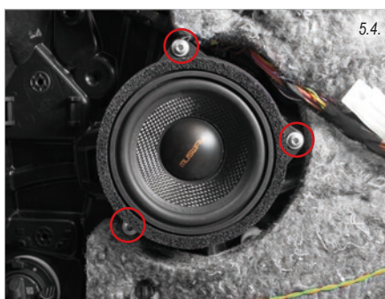
Now mount the Musway speaker with the screws
