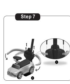
7.Assemble the safety bar into the backrest by the thumb latch, then insert the safety bar into the hole of safety bar fixed part.
