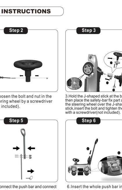
tube with two bolts and nuts as a whole push bar, then take out the snap ring in the end of the tube for standby.
