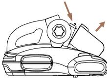
1. Push the dust cup release button and remove the dust cup.
