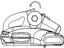
1. Rotate the right lid of the cyclone cup counterclockwise to open it and remove the filter from the cyclone cup.
