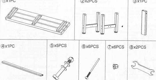
**Step1.** First the transverse pipe 4 and 3 reinforcing tube fixed by 6, and then the ② foot fixed by ⑥, all according to the figure aligned with the C-shaped slot hole, with the cross screw batch after tightening the (7) into the hole.
