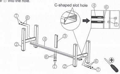
Step 2. First screw the screw washer and nut out, and then put the ① panel flat according to the figure, the first step installed the tripod into the panel ① slot, with the ⑤ in turn according to the figure to load the hole, and with spanner ⑧ tightening, set complete.2. First screw the screw meson and nut out, and then put the 1 panel flat according to the figure, the first step installed the tripod into the panel (1) slot, with the (5) in
