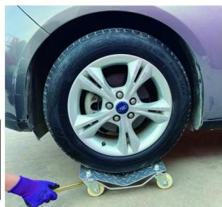
Adjust the caster orientation before pushing the cart.
