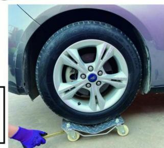
Adjust the caster orientation before pushing the cart.
