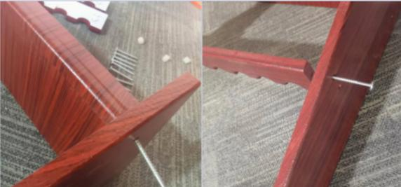
3. Secure the base plate with screws, pay attention to the fact that the raised side of the base plate faces down.
