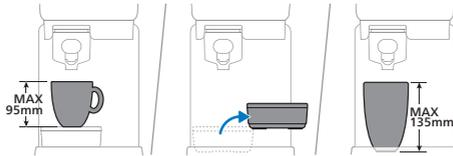
You can remove the drip tray to create extra space to place taller cups or glasses. If the drip tray is removed you can place a cup with a height of up to 135mm.
