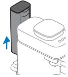
**3** Remove the water tank from the machine.
