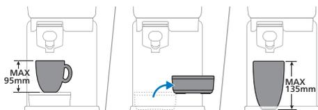
You can place a cup with a height of up to 95mm when the drip tray is placed. You can remove the drip tray to create extra space to place taller cups or glasses. If the drip tray is removed you can place a cup with a height of up to 135mm.
