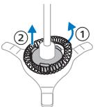
2 Remove the lid and then remove the whisk holder from the milk frother.
