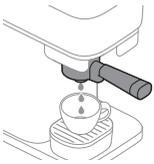
**7** The machine heats up and starts rinsing water from the coffee spout into the cup. The Intensity boost button will continue to blink slowly during this process.
