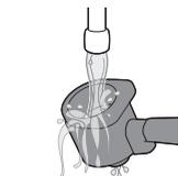
**Warning:** Do not use any sharp objects to empty or clean the portafilter, as this may damage the sealing surfaces.
