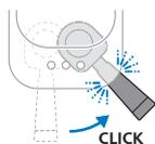
The direct start function allows you to switch on your machine and brew delicious coffee easily. There is no on/off button. Simply press the button of the drink you want to brew. Then move the portafilter to the right to start the grinding and the brewing process.
