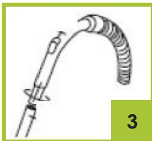
4. To connect the tube with pads, insert the smaller pipe tip to the pad and turn to make the strong connection.
