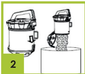
3. Open the top part of the tank and remove filters.
