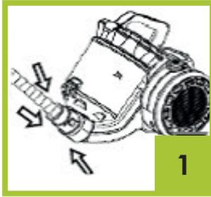
2. To take the hose out, press two buttons and remove it.
