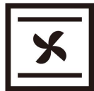
Fan, bottom and top heaters on
