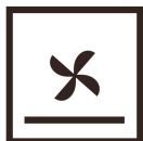
Fan and bottom heater on
