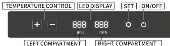
**Note:** the right compartment is on the side where the compressor is.
