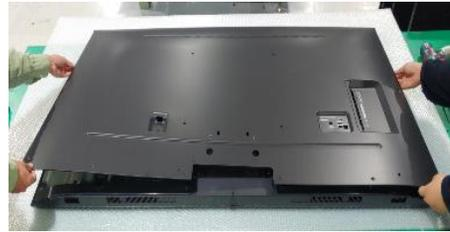
Once removed, this will expose the accessible electronic units (PCBs) which can now be easily removed with hand and screw driver.
