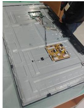
LCD (together with their casing) is only left after all other parts like electronic units have been removed.
