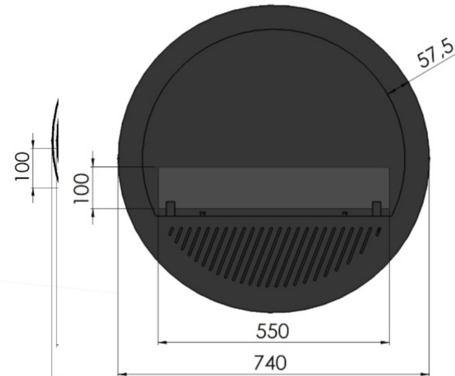
Type - To be installed in a round recess (about Ø690mm).
