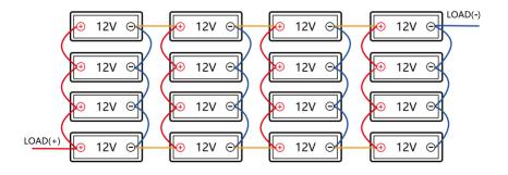
Taking a 12V 50Ah battery as an example, first, four such batteries in parallel form a 12V 200Ah pack. Then, four of these packs in series produce a 48V 200Ah battery pack.
