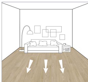
For plank and tiles designs, sheets should be installed in the same direction.
