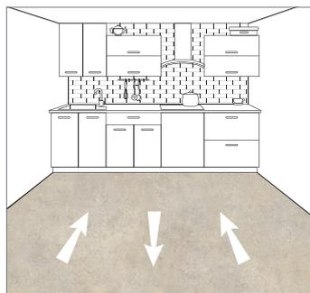
For most all-over designs, alternate sheets should be installed in opposite directions. Check design specifications before you start.
