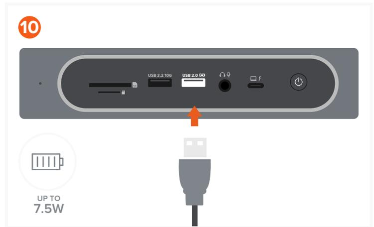
Use the USB-A 2.0 port for charging a USB device – up to 7.5W.
