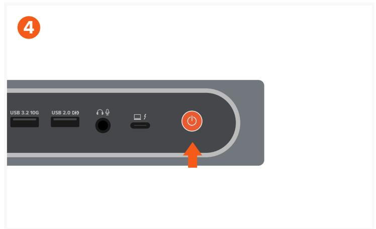
4 After connecting the dock, press the power button on the front of the dock to turn it on. The power LED will change from white to green once fully connected to host device
