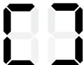
To activate the open windows detection function, hold the timer button on the control panel for 5 seconds. The buzzer sounds twice to indicate that the function is turned on, and the buzzer sounds once to indicate that the function is turned off.
