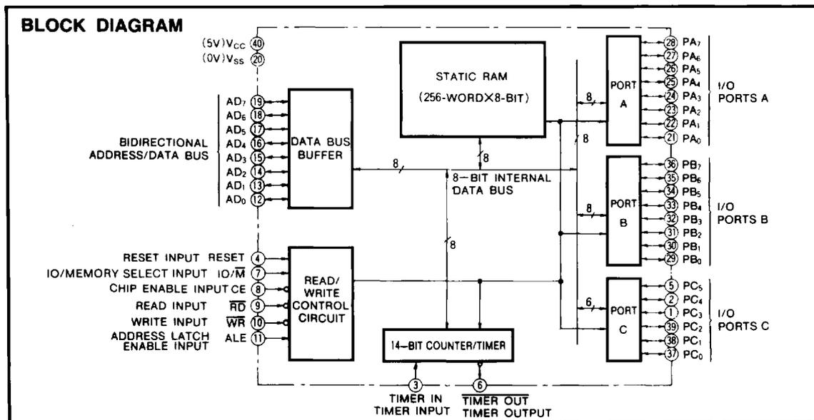
2048-BIT STATIC RAM WITH I/O PORTS AND TIMER
