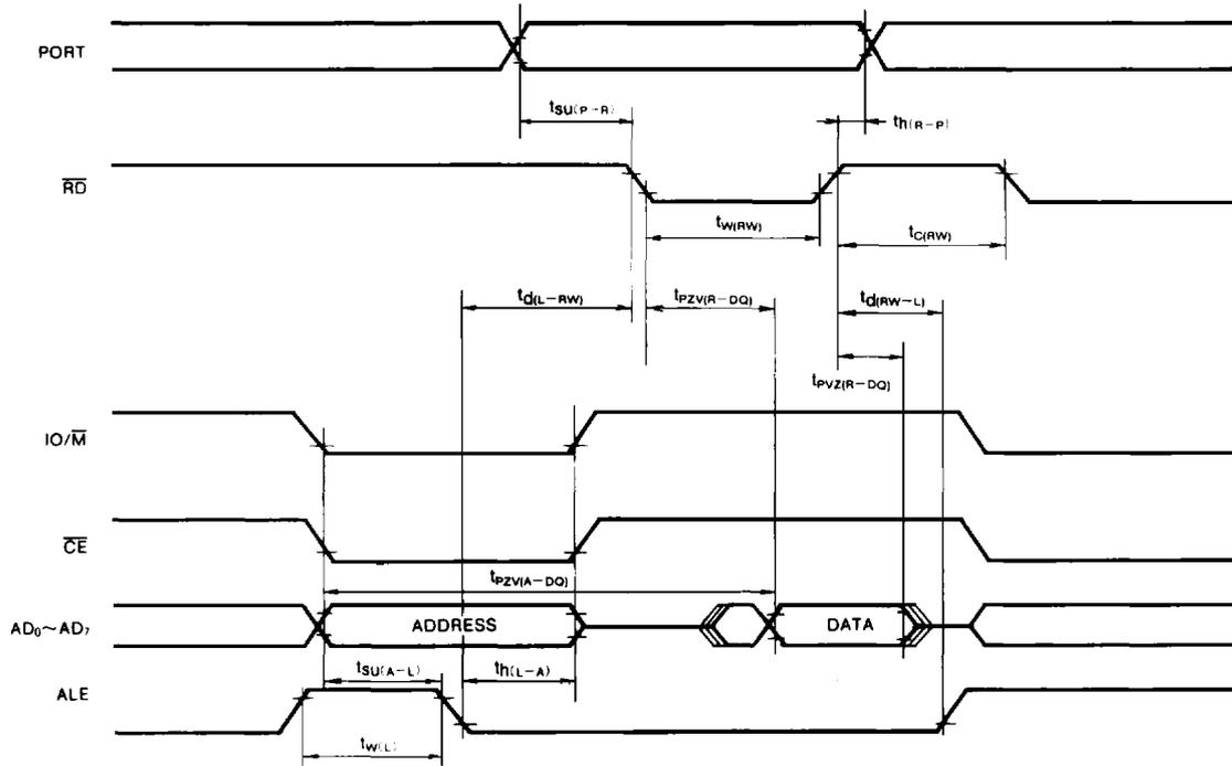
2048-BIT STATIC RAM WITH I/O PORTS AND TIMER
