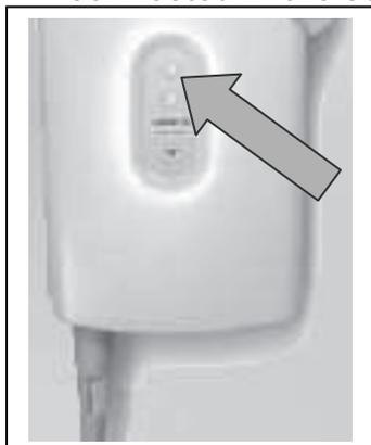
When the batteries are recharging there will burn a yellow light on the upper LED.
