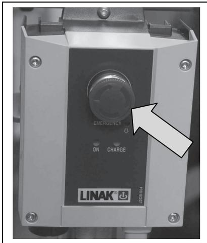
In emergencies, and during assembly and disassembly, the emergency stop is activated by pressing the red button on the control box.
