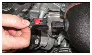
3. Unlock the red locking tab on the air temperature sensor electrical connection, then depress the locking lever and pull apart the temperature sensor electrical connection.
