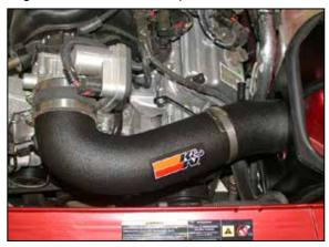
18. Install the K&N<sup>®</sup> intake tube into the throttle body and onto the saddle clamp as shown, then secure with the hose clamps provided.
