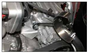
13. Using the provided spacer, install the tube mounting bracket assembly onto the engine as shown.
