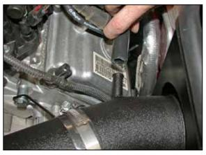
19. Install the provided crank case vent hose onto the vent port on the valve cover then install the vent hose onto the  $K\&N^{\mbox{\ensuremath{\$}}}$  intake tube.
