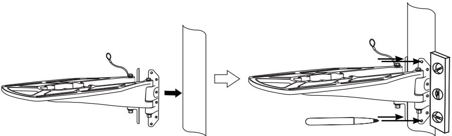
**4** Using a 3/16" drill bit, drill all the marked holes.
