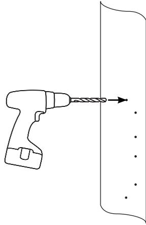
**5** Use a hole saw to drill a hole for the cables. Be sure to drill in the center of the mast.
