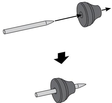
**7** Insert the rubber grommet into the hole you drilled for the cables.
