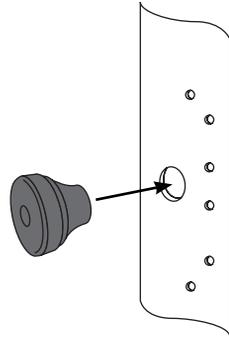
**8** Put some marine adhesive sealant into the holes. Do not apply too much sealant.
