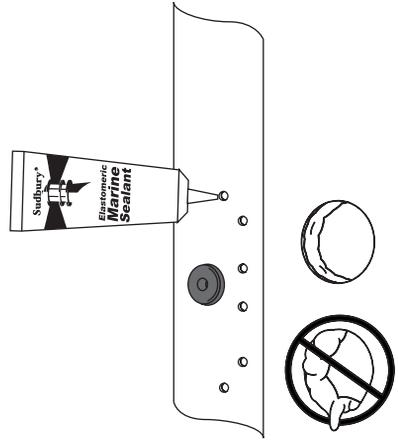
**9** Insert the black nylon shoulder washers into the correct holes on the mast mount feet. Use the supplied rivets to secure the mast mount to the mast.
