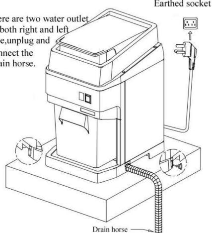
3. Lift up the top lid and load ice cubes into hopper
