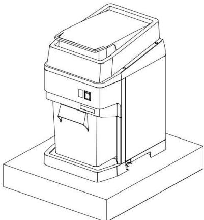
2. Plug in the socket and connect the drain horse.
