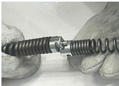
Connect the soft shaft with drills
