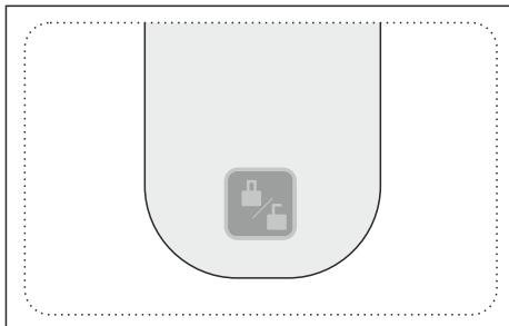
The table is equipped with a safety switch located on the remote control. After pressing and holding for 3 seconds, the table raising and lowering function is blocked. To unlock the function, hold the button down again for another 3 seconds.
