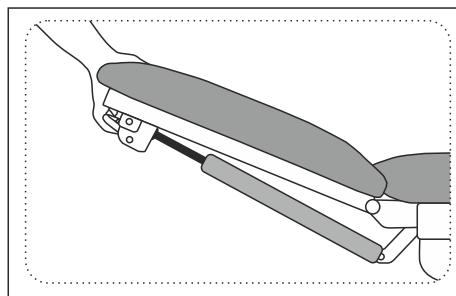
After releasing the lever, the headrest in the desired position can be adjusted.
