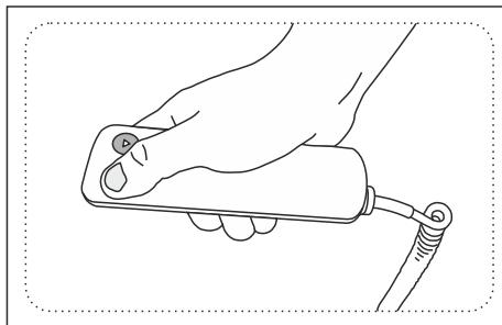
Control takes place by pressing the buttons marked with arrows – up/down.
