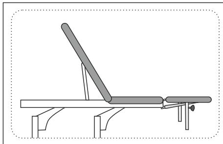
The rear section of the seat is adjusted using a Rastomat mechanism. Raise the segment to the selected position, the mechanism will lock automatically.
