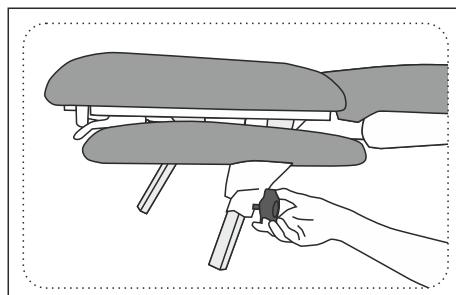
To lower the armrest down, unscrew the knob counterclockwise and then adjust the height to the required position. Then tighten the knob clockwise.
