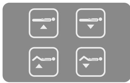
In selected options, in addition to adjusting the total height of the tabletop, it is possible to adjust the angle of the bed in the range of 0-25°. The control is performed by pressing one of the buttons marked with up/down arrows.
