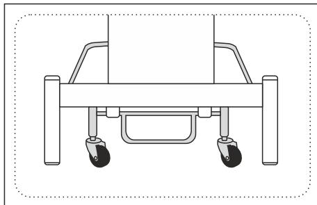
The driving system is activated by lifting the table using the foot lever. By pressing the lever down, the table supported on wheels can be moved. To lock the table in the selected position, lower the table onto the feet by lifting the lever to the upper position.
