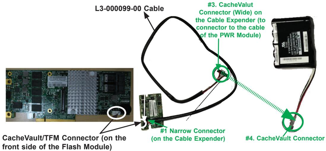
2. Connect the wide CacheVault/TFM connector (#3) on the L3-000099-00 Cable Expander to the CacheVault connector (#4) on the end of the cable attached to the Power Module as shown on the third picture above.
