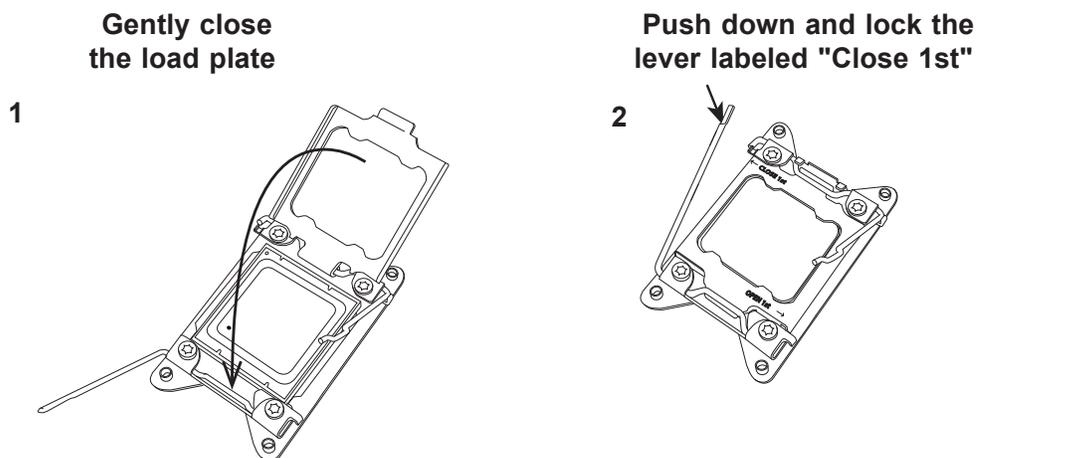
8. Close the load plate with the CPU inside the socket. Lock the lever labeled "Close 1st" first, then lock the lever labeled "Open 1st" second. Using your thumb, gently push the load levers down to the lever locks.
