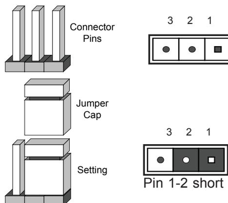
**Note:** On two-pin jumpers, "closed" means the jumper is on the pins, and "open" means the jumper is off them.
