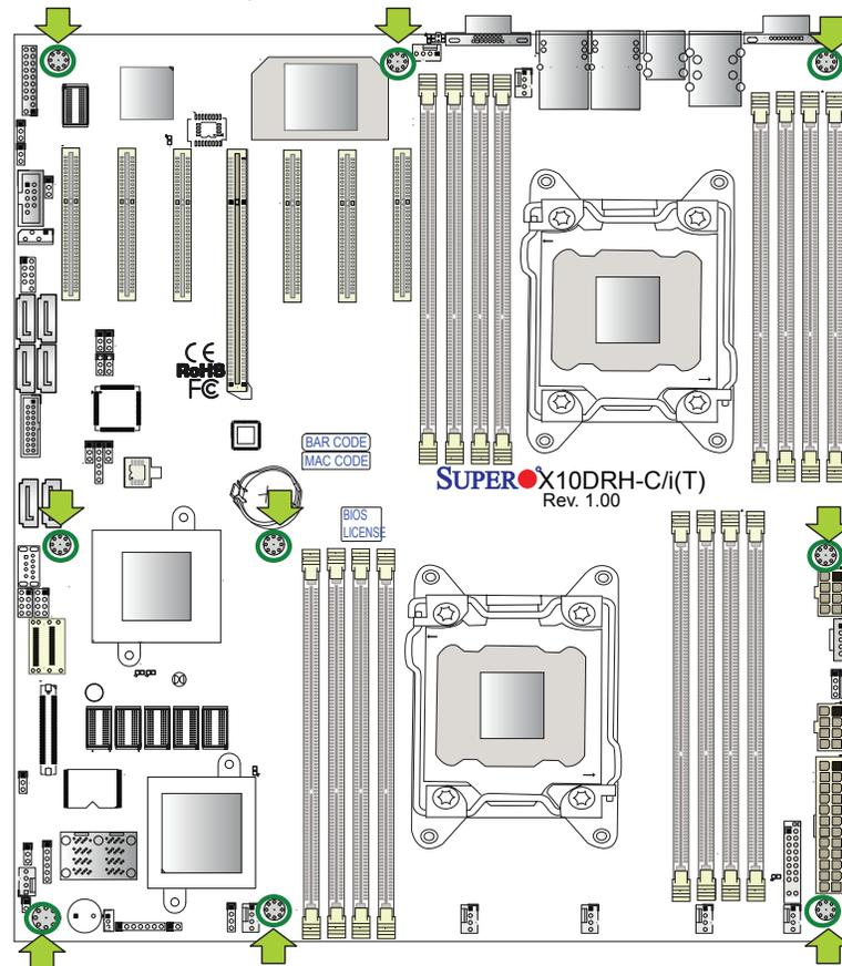
**Caution:** 1) To avoid damaging the motherboard and its components, do not use a force greater than 8 lb/inch on each mounting screw during motherboard installation. 2) Some components are very close to the mounting holes. Please use caution to prevent damage to these components when installing the motherboard to the chassis.
