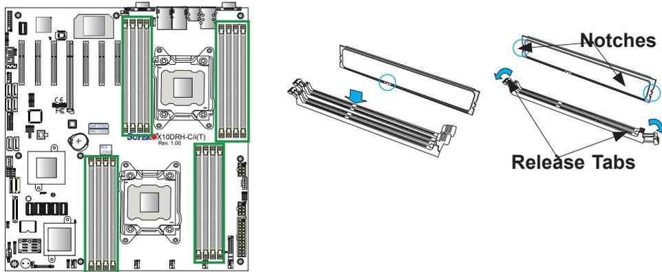
3. Align the key of the DIMM module with the receptive point on the memory slot.
