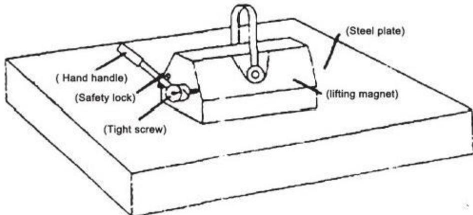
In the first step, place the permanent magnetic lifter in the center of the steel.
