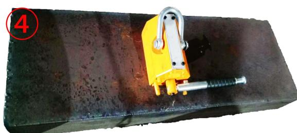
The last step, after confirming that the permanent magnetic lifter is closed, remove the permanent magnetic lifter and store it in a dry place to prevent rust.
