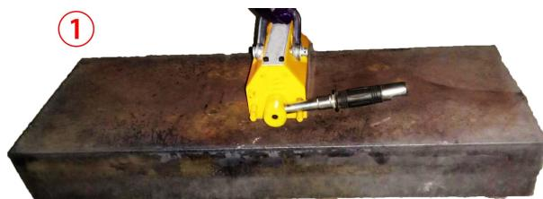
The second step, press the handle button and turn the handle from OFF to ON, and the handle can only be released after the safety lock is locked. It is strictly forbidden to use it with no load or overload.
