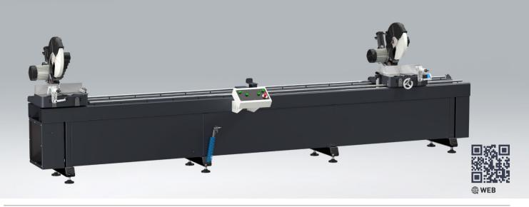
The GEMINI II M machine is a double-head aluminum and PVC cutting machine. It can cut profiles up to 4000 mm in a single operation. Its robust chassis ensures a long service life, while its 400 mm saw blade allows for the precise cutting of large-sized profiles.
