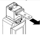
Thanks to recent mechanical improvement the strong interlocking system guarantees a maximum actuator holding force of 1100 N (head 96)
