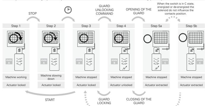
The GUARD CLOSING with de-energized solenoid brings the switch back in B state and then in A state in quick sequence
