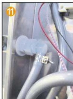
11 Connect the water outlet connector and hand spray Seat joint
