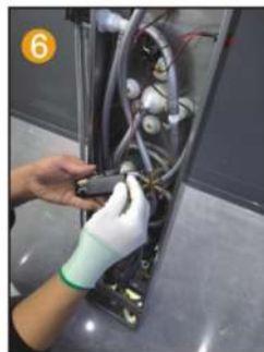
6 Install 2 No. 5 batteries to chargePool box
