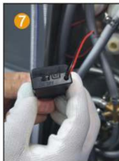
7 Point the switch of the battery box towards ON
