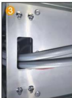
3 Fix the motherboard and top spray with 4 pairs of M6 screws and nuts
