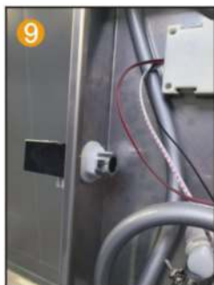
9 Spray socket with hexagonal nut handle Fixed on the panel
