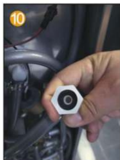
10 Put the 4-point rubber into the hand spray inside the joint of the seat
