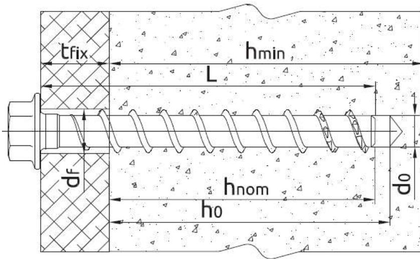
**R-HLX-CS - Installed screw**
