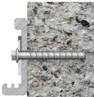
6. Correctly installed screw with a sealing ring filled with resin.
