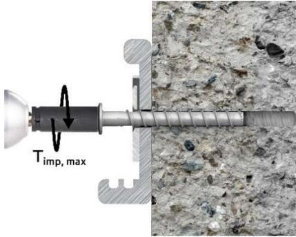
3. Place the sealing ring on the fixture. Screw the concrete screw into the hole using an impact wrench and an appropriate impact socket. Tighten until the element is pressed to the surface. Installation using any impact wrench with a tangential impact.
