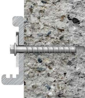
4. Finish screwing in when the screw head and the ring are in contact with the fastened element/substrate. The screw head must not be damaged.
