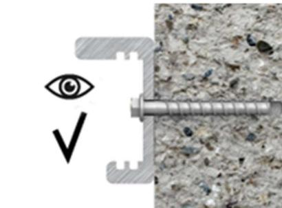
4. Finish screwing when the screw head is in full contact with the fastened element/substrate. The screw head must not be damaged.
