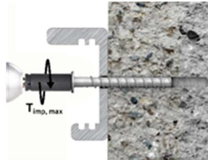
3. Screw the concrete screw into the hole with an impact wrench and a suitable impact socket. Tighten until the fixture is clamped to the substrate.
