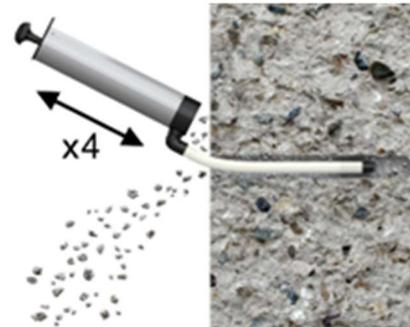
2. Clean the hole (blow dust at least 4 times with the hand pump). When using a dust-free drill bit (1b), it is not necessary to clean the hole.
