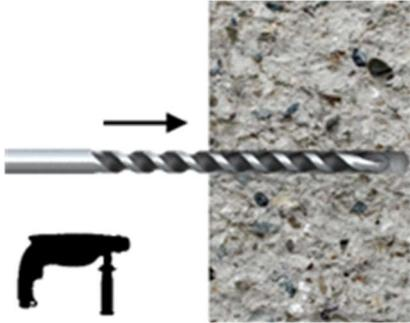
1. Drill the hole with a hammer drill (1a) or a dust-free drill (1b) to the required depth according to the table.
