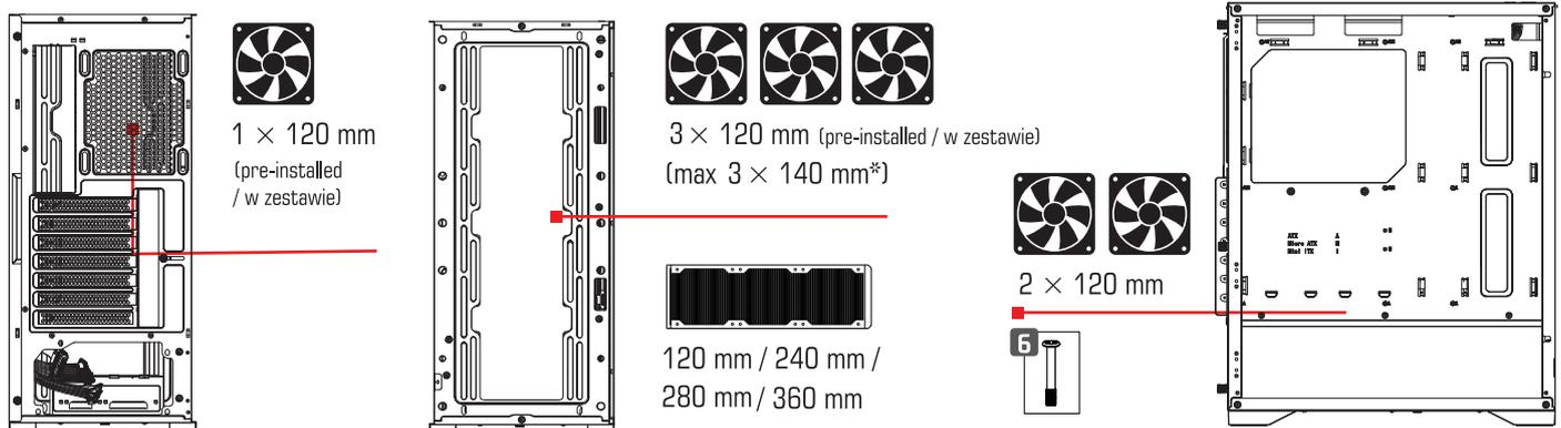
\* Installing 3 x 140 mm fans on the front of the case is possible only from the inside of the case.
