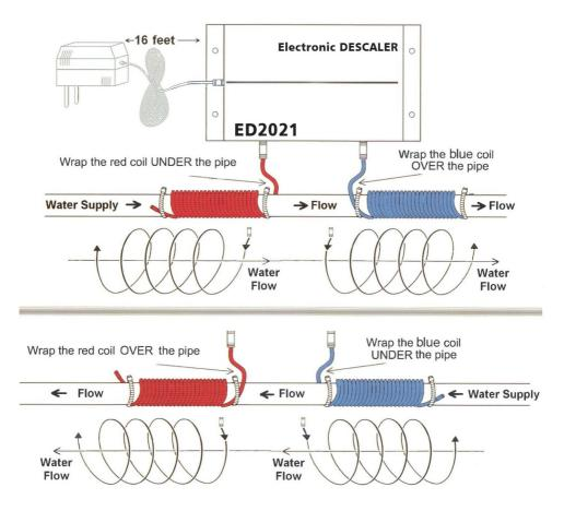
Wrap the full length of each coil around the pipe in their respective directions. Make sure the coils are wrapped snug against each other, leaving no space between the coils on each wrap.
