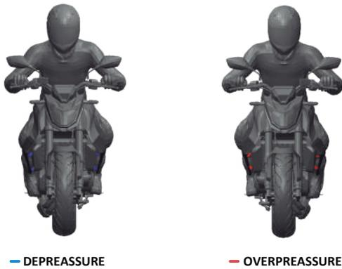
Due to its angles and frontal surface, it creates an overpressure on the top of the spoiler. The turbulence create below, generates a difference of pressure between the upper and lower part of the spoiler. Which ultimately generates the aerodynamic downforce.
