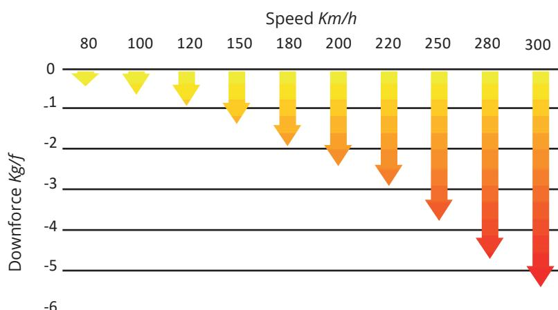
The Downforce that the spoilers generates raises potentially as the speed increases, at top speed we get 3,2 Kg/f.
