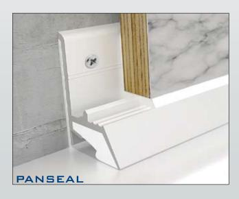
The sealant is concealed and protected inside the trim while a silicone bond-breaker tape releases the sealant off the trim for flexibility.
