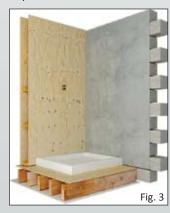
Timber joist shrinkage is common in new buildings causing the joint between the ledge & wall to expand.
