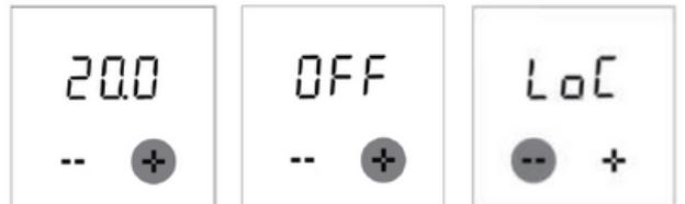
When the frost protection function is activated, the thermostat will maintain the floor temperature at 5°C in the off state.
