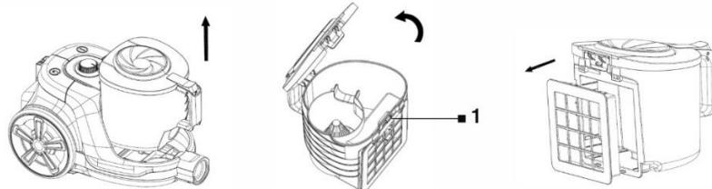
11. Press the latch to open the tray (1) and empty the dirt and dust.
