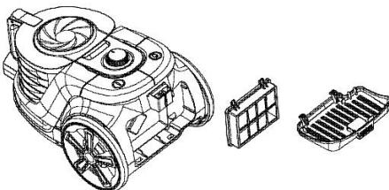
14. For rough cleaning, gently knock the dirt from the HEPA filter into the waste bin.
