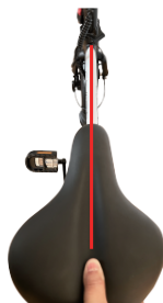
16. Before riding, you must check whether the seat head and the frame are aligned in a straight line, and whether the seat is loose.
