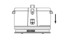
3 After cleaning, cover the dirty water tank with the lid, then install the dirty water tank back into the machine until you hear a "click" sound, indicating it is properly installed.
