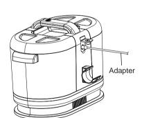
2 As shown in the figure above, plug the adapter charging port into the charging terminal of the machine, and then the adapter can be charged normally when powered on, the red light will flash when charging, and the blue light will be on when fully charged.
