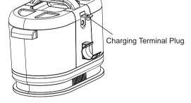
Grasp the arc-shaped protrusion at the bottom of the charging terminal plug, then remove the charging terminal as shown in the diagram.
