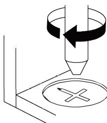
**EN**\_Turn cam lock clockwise to tighten.
