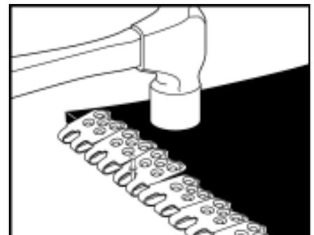
6. Using a 2 lb. (0.9 kg) hammer, tap top plates into the belt.
