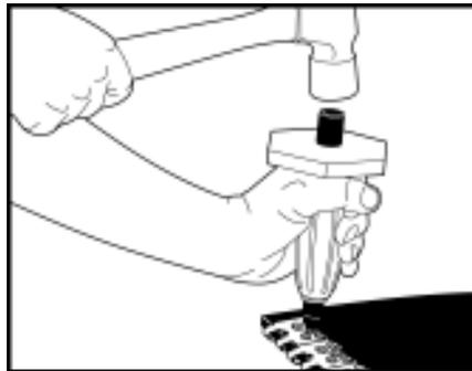
10. Turn belt over and place on hard surface. Set rivets using a 2 lb. (0.9 kg) hammer and R5S rivet set tool. Belt should pucker around fastener edges.
