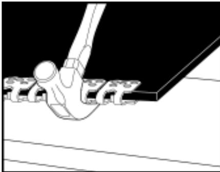
9. Remove nails securing the belt. Pry belt from wooden board. Pilot nails should remain in the board, knock off any still attached.
