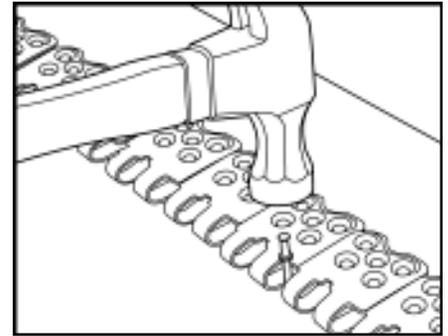
3. Place fastener strip on a wooden board, Flexco stamp facing up. Drive three nails between fastener loops to secure fastener.
