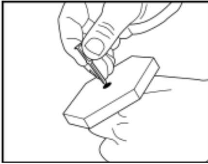
7. Remove drive rod from SR50. Load tool with rivets. Replace drive rod.
