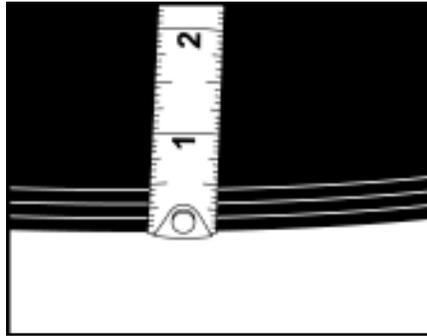
2. Measure belt thickness from cut edge using gauge or tape measure. Select correct size SR rivets for your belt thickness.
