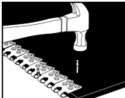
5. Nail belt to wooden board to secure belt.
