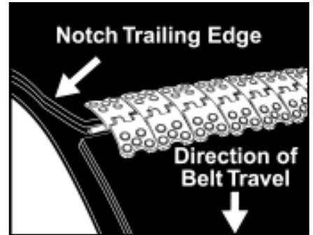
11. Repeat steps 1-10 on other belt end. Bring belt ends together and insert hinge pin. Notch trailing edge of belt only. Splice is complete.
