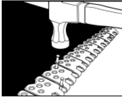
Alternative: Rivets can be driven using a 2 lb. (0.9 kg) hammer, without using the SR50 tool. The SR50 is the safer method.
