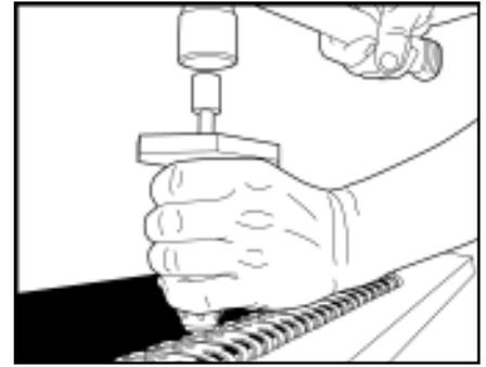
8. Using a 2 lb. (0.9 kg) hammer, drive rivets into the middle fastener plate, then each end plate. Drive rivets in remaining plates.
