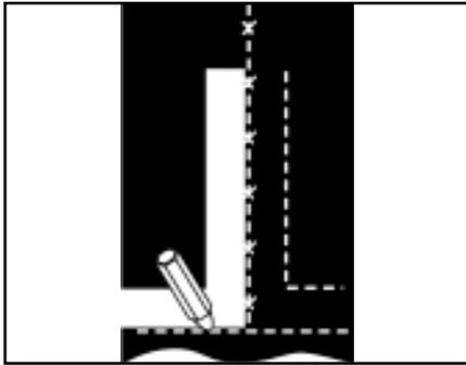
1. Square belt using centerline method. Cut belt 4" (100 mm) behind old splice using a utility knife or Flexco belt cutting tool.
