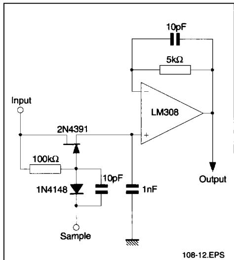
**FAST SUMMING AMPLIFIER WITH LOW INPUT CURRENT**
