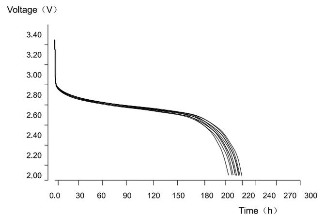
\*Delivery Capacity is dependent on the applied load, operating temperature and cut-off voltage. Please refer to the charts and discharge data shown for examples of the energy/service life that the battery will provide for various load conditions.
