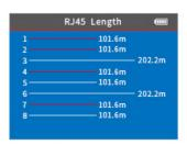
Utilises TDR to accurately measure cable length with visual length graphics and provide distance to fault information.
