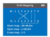
TDR helps to pinpoint where cabling faults occur. This speeds up fault finding as well as minimising disruption and potential damage to fixtures and fixings.
