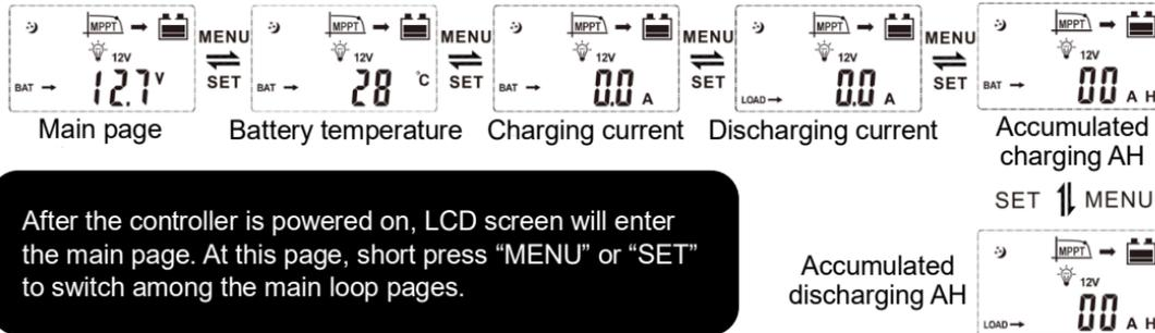
After the controller is powered on, LCD screen will enter the main page. At this page, short press "MENU" or "SET" to switch among the main loop pages.
