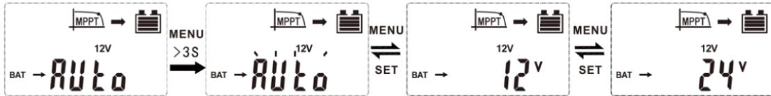
After entering setting pages, switch to the system voltage page, long press for "MENU" 3 seconds until the "auto" starts to flash. Then short press "MENU" or "SET" to turn the system voltage 12V or 24V.
