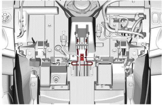
Driver seat hidden for clarity 2. Install slider [P2].
