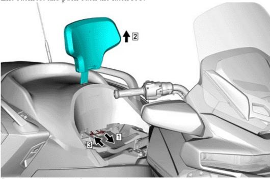
Step 1:. Pull latch rod forward to unlock Step 2:. Lift backrest Step 3:. Push back the latch rod
