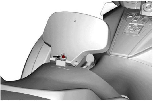
Backrest Removal Lift the driver's seat and pull latch rodforward to unlock the backrest. Lift backrest and push back the latch rod.
