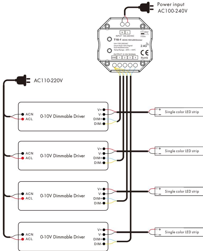
Note: We recommend the number of LED drivers connected to 0/1-10V dimmer (each channel) does not exceed 20 pieces, The maximum length of the wires from dimmer to LED driver should be no more than 30 meters.
